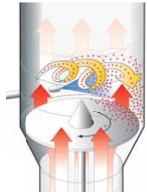
Tangential spray in the rotor insert
